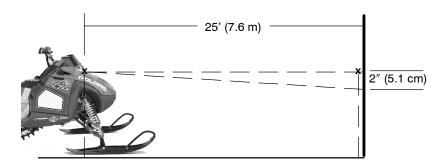
The headlight may be adjusted for vertical aim using the following procedure:
